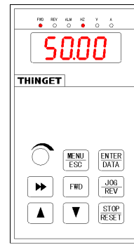
Fig. C Running status, display the running parameters
